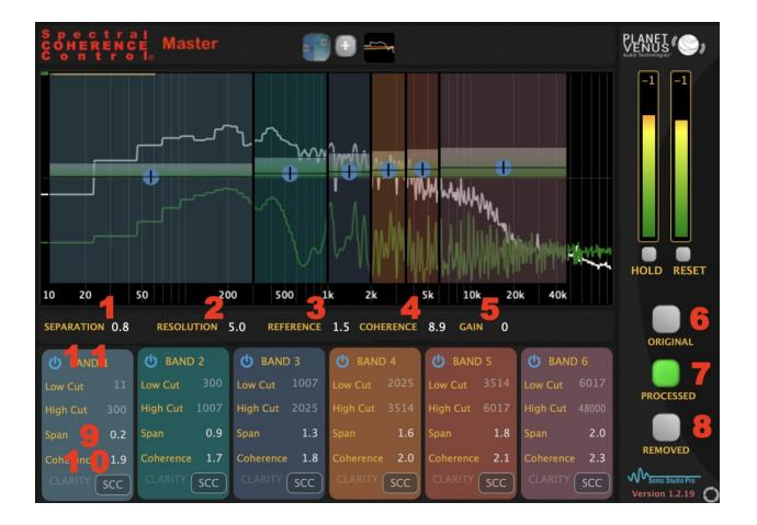
• Figure 2 Spectral Coherence Control <sup>®</sup> Graphical User Interface window
